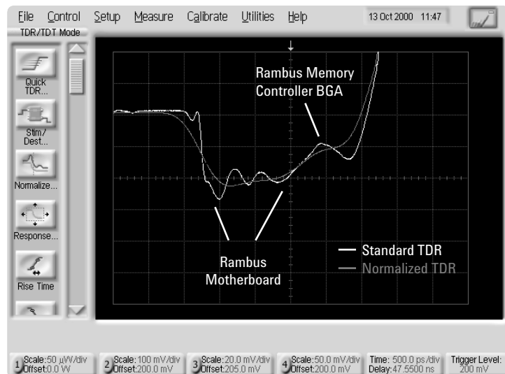
Figure 3. Probing a Rambus motherboard from the RIMM connector side
